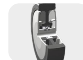
Construction of wheel: ball bearing, sealed
